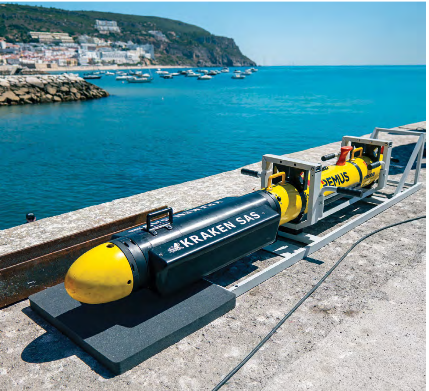
Kraken SAS integrated onto REMUS (photo credit: Kraken Robotics).
