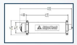
The BRT6000 Burn Wire Activator/ Acoustic Transponder is a reliable and versatile mooring instrument. The BRT6000 is made entirely of Nickel Aluminum Bronze for superior corrosion resistance and deep deployment. Acoustic status reply includes both tilt, Activation Confirmation and optional inputs. The command structure used has been proven in the toughest acoustic environments anywhere. Deployments up to two years on alkaline batteries.
