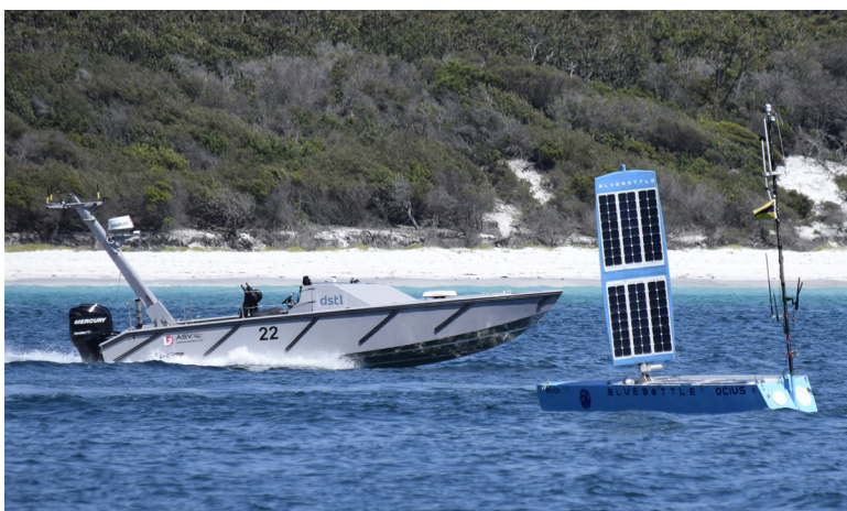
Left: The Maritime Autonomy Surface Testbed from the Defence Science and Technology Laboratory (UK), and Bluebottle from OCIUS (right), at Exercise Autonomous Warrior 2018 held at HMAS Creswell, Jervis Bay. Image courtesy of the Department of Defence.
