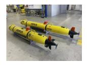
The REMUS 100S is a specialised evolution of the highly successful, man portable REMUS 100 system configured specifically for hydrographic and offshore surveys. Supplied as one element of the unmanned systems toolbox for RAN Project SEA1770 Rapid Environmental Assessment, the REMUS100S enables high accuracy seafloor surveys in support of amphibious or other operations.
