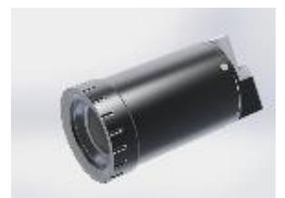
with Kowa 6mm lens. The application was for mounting the cameras on a pipeline crawler for long-distance inspection of partly flooded pipelines. Both the housings and associated junction tube needed to be as space efficient as possible. Both were designed to be waterproof to 100m depth and a hard-anodised finish on both items was required.
