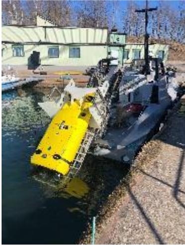
Saab's unique Multi-Shot Mine Neutralisation System (MuMNS) is a powerful, reliable and adaptable vehicle that can be used in a variety of different roles, including live operational mine clearance, peacetime operations against historical ordnance, mine investigation and underwater demolitions. The system is effective against a complete range of underwater targets: mines (ground, moored, floating and drifting), depth charges, torpedoes and IEDs.
