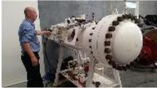
The existing hydrostatic pressure test capability at the BlueZone Perth facility has been improved with the addition of the capability for live testing of cable assemblies and Electric Fly Leads (EFLs). Customer-specified test cycles including live testing for continuity, isolation and insulation at pressure up to 3000psi (2000 metres of seawater).
