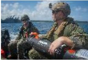
The AUV can perform pre-programmed missions autonomously as they are equipped with Seebyte Neptune software. The software can make and execute its own decisions during a mission.
