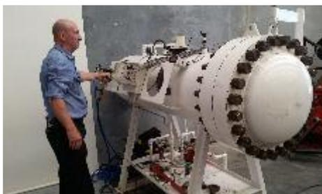
Due to customer demand, BlueZone has relocated a 2000m rated hydrostatic pressure test chamber from workshops in Melbourne to Bibra Lake in Perth. General Manager Perth, Mark Musarra, said that there had already been a high demand for hydrostatic pressure testing services. "We have completed two customer jobs this week," said Mark, "and are very pleased to have the test chamber in Perth to offer rapid turnaround for our West Australian customers."
