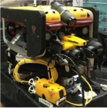
An ingenious idea from Saab Seaeye customer, Stinger Technology, has found a way to penetrate the labyrinth inside offshore production tanks in search of environmental contaminants prior to decommissioning. They managed to squeeze a unique underwater robotic systems configuration loaded with sampling technology through a 150 cm square hatch to search the tank's internal maze of baffles, and navigate along 25.5 cm diameter pipe-runs of curves and bends.
