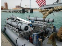
In a recent study a REMUS AUV outfitted with a bathyphotometer module was used to examine the fluctuations of bioluminescence in relation to the physical dynamics in the working harbour at San Diego. The study demonstrated the utility of AUVs in measuring bioluminescence and future uses could be as a means of passive threat detection of surface and subsurface vehicles and swimmer tracks.
