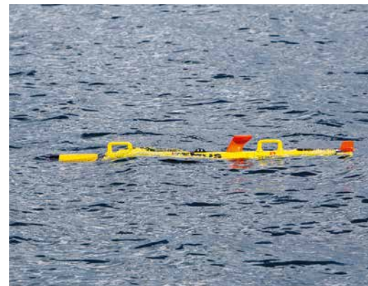
REMUS 100 returns to the surface after completing sonar and oceanographic surveys of the sea floor during Autonomous Warrior 2018. (CoA / Justin Brown)
