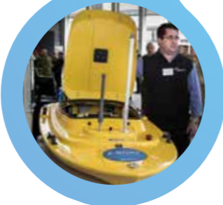
The Teledyne OceanScience Z-Boat is a rugged and capable platform that is ideal for river discharge measurement using an ADCP.
