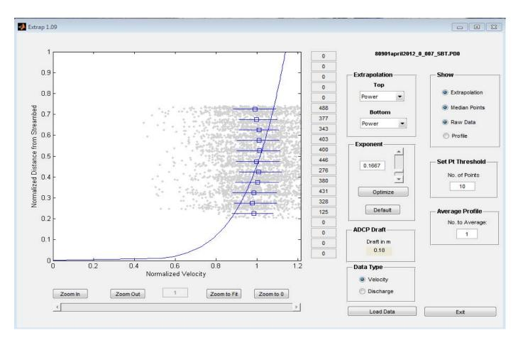
This example indicates that the defaults of power curve top and bottom aren't such a good fit
