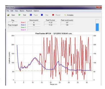
Beam 1 faulty after firmware upgrade
