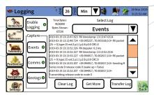
**Geotagging feature**, when enabled, allows a geographic location to be recorded along with the time and other details for all important acoustic events. Now it is easy to track exactly when and where an acoustic release was ranged to or triggered.
