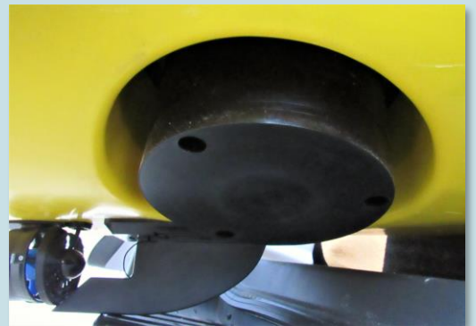
The transducer of the SUBPRO 2545 mounted into the hull of the USV.
