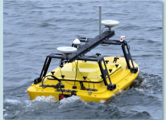
The SUBPRO 2545 in operation, integrated into an unmanned surface vehicle (USV).
