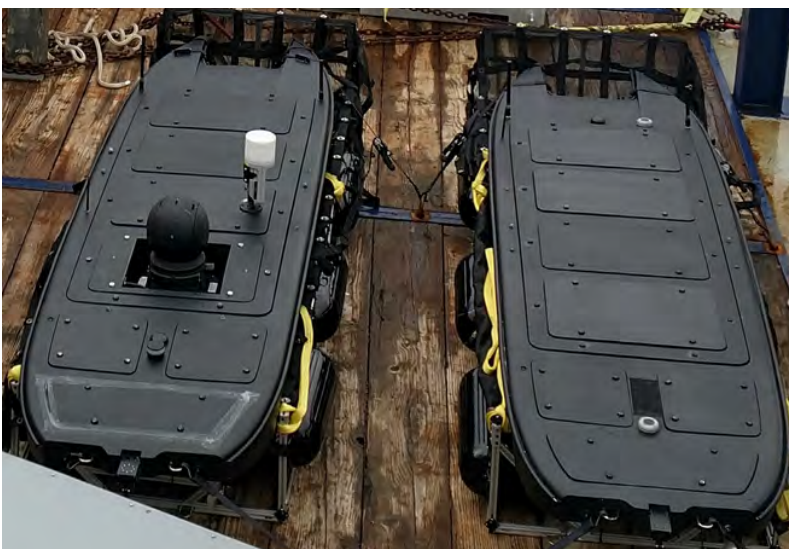
This shows several MANTAS T12 unmanned surface vehicles before deployment during an offshore exercise. Photo courtesy of Maritime Tactical Systems, Inc.
