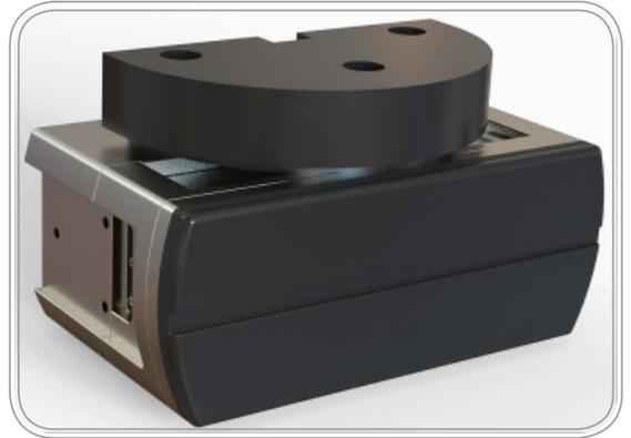
The SeaBat F30 is a High-Resolution Forward-Looking Sonar System designed specifically for 12 ¾ inch (approx. 324mm) AUVs/UUVs. The SeaBat F30 operates at 200 kHz or 635 kHz illuminating a wide, 120° horizontal sector ahead of the Sonar Head Assembly. The high frequency 635 kHz provides high-resolution classification functionality, whereas the lower frequency 200 kHz provides long-range detection capability.
