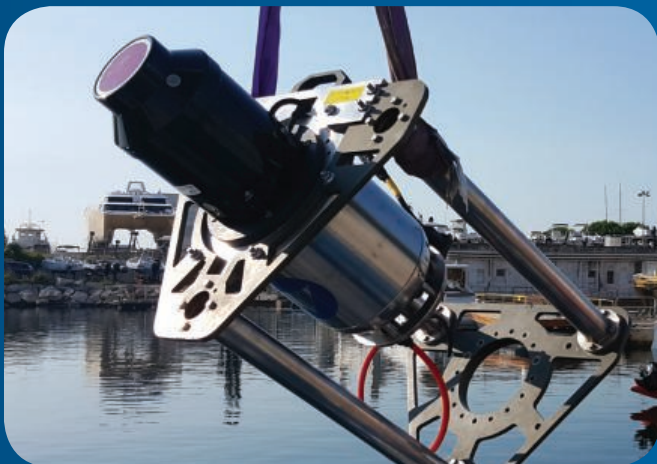
Teledyne RDI Pioneer 600 kHz DVL fitted with iXblue PHINS 6000 inertial navigation system
